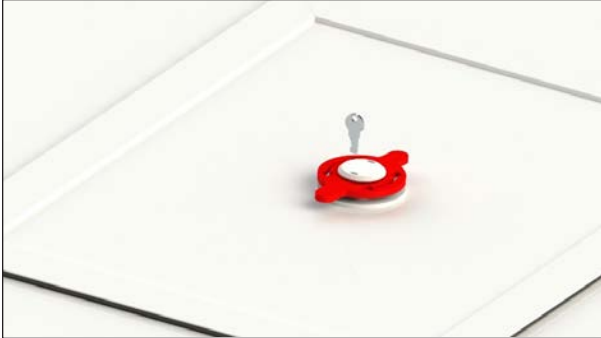
FIGURE 108: USE THE KEY INSIDE THE SLOT
